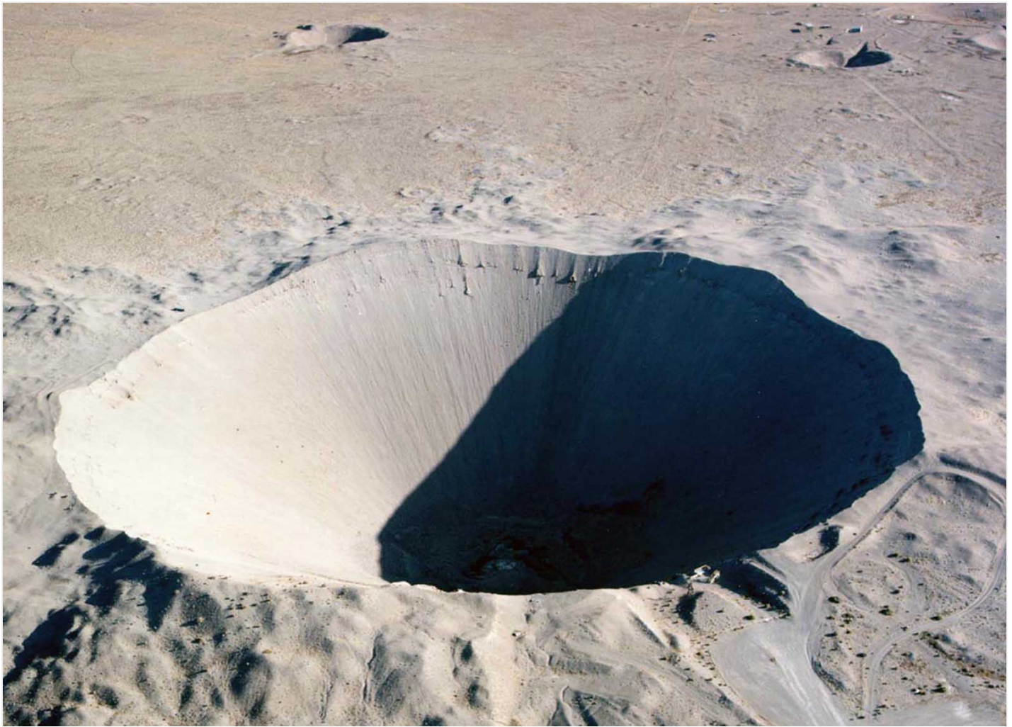
Sedan Crater was formed when a 100-kiloton explosive buried under 635 feet of desert alluvium was fired at the Nevada Test Site on July 6, 1962, displacing 12 million tons of earth. The crater is 320 feet deep and 1,280 feet in diameter.
